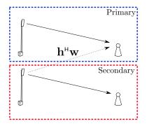
With the knowledge of the SNR, the secondary BS designs a precoder w which is orthogonal to the sub-space spanned by hh<sup>H</sup>.
