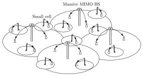
Every device estimates its received interference covariance matrix and precodes (partially) orthogonally to the dominating interference subspace.
